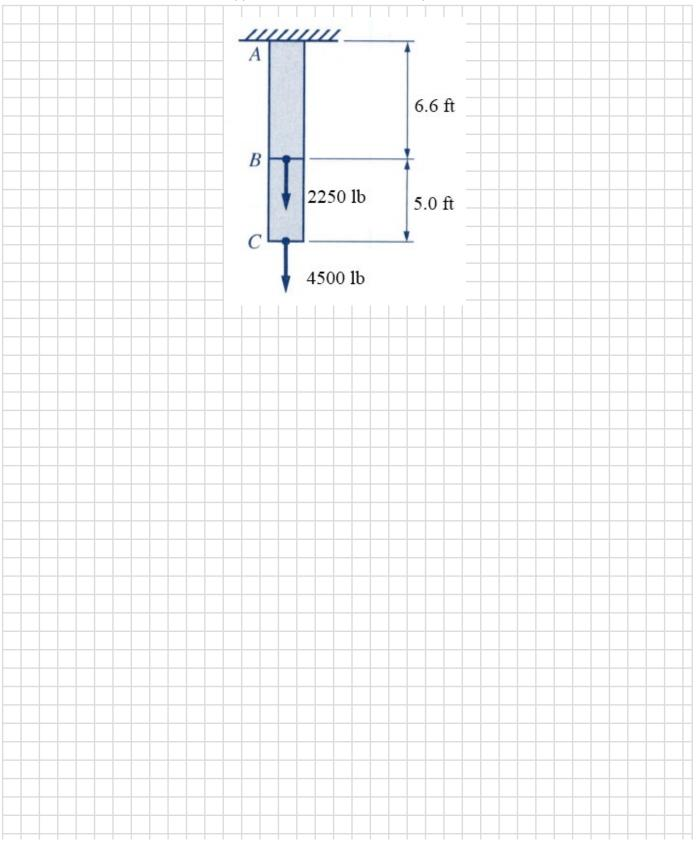
See Fig. P10-10. Determine the total elongation of the steel eye bar BC of 0.4 in. (10-mm) diameter due to the load P = 1800 lb (8 kN). The modulus of elasticity of steel is E= 30,460 ksi (210 GPa).
